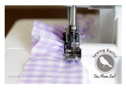
For me, gathering on the sewing machine is tedious and frustrating but gathering on the serger is fast and easy. Gathering is made possible by the serger's differential feed. A setting higher than 1.0 will cause the fabric to 'bunch up.'
